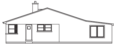
02 EXISTING NORTH ELEVATION (RIGHT SIDE) SCALE: 1/8"=1'-0"
