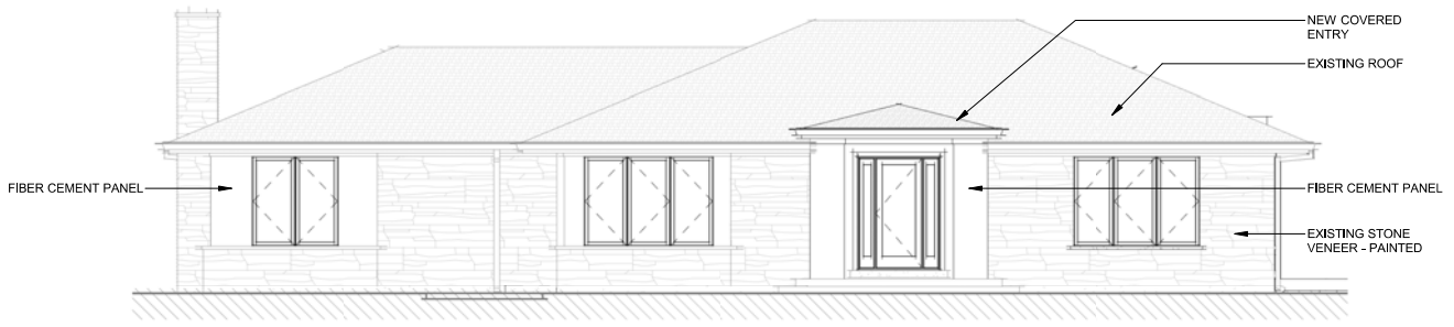
① FRONT (EAST) ELEVATION 1/8" = 1'-0"
